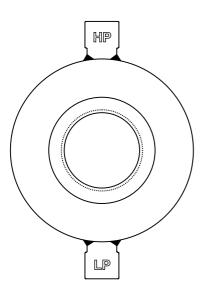
Due to its small thickness, the single ring orifice carrier is often a cost effective solution, and may be manufactured in a wide range of exotic materials including Hastelloy<sup>®</sup>, Monel<sup>®</sup>, Duplex Stainless Steel, Inconel<sup>®</sup> and Incoloy<sup>®</sup>
